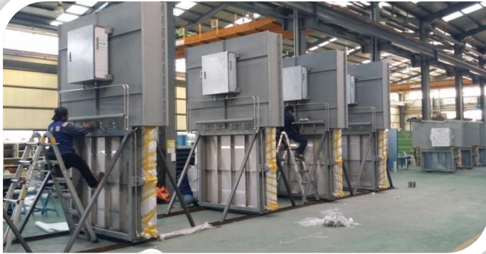
SLIDE GATE (CYLINDER TYPE)
